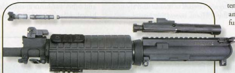
The Gas/Piston Carbine can be field stripped of its moving gas-system components (the piston and operating rod) in a matter of seconds.
