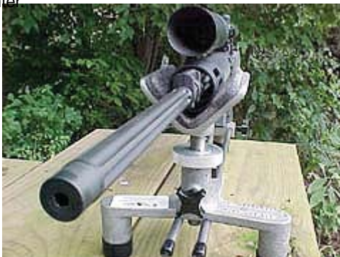
The heart of the Bushmaster Varminter's amazing accuracy is the beautifully designed and executed barrel. The 24" chrome-moly barrel is fluted along its entire length, with the diameter stepping down from a full 1" inside the aluminum handguard to .745" forward of the gas block.
