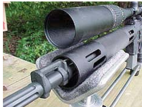
The heart of the Bushmaster Varminter's amazing accuracy is the beautifully designed and executed barrel. The 24" chrome-moly barrel is fluted along its entire length, with the diameter stepping down from a full 1" inside the aluminum handguard to .745" forward of the gas block.
