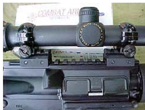
The Varminter is fitted with a comfortable and practical soft pistol grip. This grip is the author's favorite for AR-15 type rifles because it is a practical aid to accuracy and it is equally comfortable to a Southpaw like the author! The Bushmaster Varminter is equipped with a "flat top" frame that will accept standard Weaver-type scope rings for a virtually inexhaustible array of sight options. Also included are two scope riser blocks for proper eye alignment and cheek-weld. The Bausch & Lomb Elite 4000 6-24x variable scope is an excellent choice for a semi-automatic tack-driver like the Varminter!
