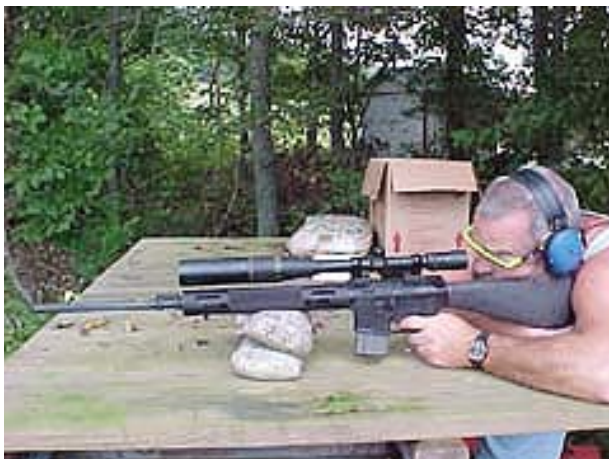
Author's bench shooting sessions with the Bushmaster Varminter left him in amazement at the accuracy potential of this excellent rifle. The Bushmaster Varminter was able to group three shots into 1/4" at 100 yards with regularity using the super-accurate Barnes VLC bullets. The worst groups shot from the bench rest were 3/4" at 100 yards! The representative 1/4" group shown above (that's a DIME shown for comparison!) show the Varminter to be one seriously accurate rifle!
